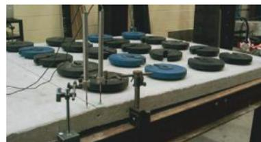
Testing at an independent laboratory measured load and freeze/thaw characteristics of a TripStop Sidewalk Assembly designed to simulate tree root invasion, soil expansion and thermal expansion.
